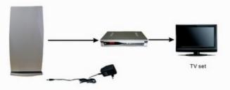
When the signal is horizontal but the antenna is vertically assembled, the signal output will be decreased by about 15dB. Also when the signal is vertical but the antenna is horizontally assembled, the signal output will be decreased by about 15dB. So you may check the signal reception effect by changing assembling polarization of antenna.
